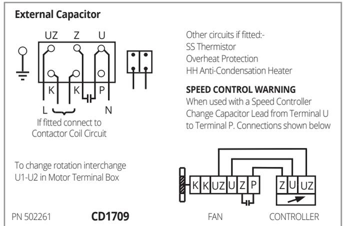
**WIRING DETAIL: SINGLE PHASE FANS WITH DUCT MOUNTED TERMINAL BOX**
