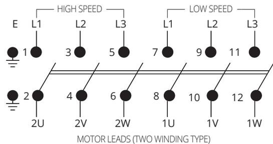
TWO SPEED MOTOR UNITS. TWO WINDING TYPE
