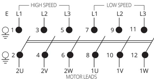
**Warning** :- Control Gear must suit Pole Change (Tapped Wound, Dahlander or Pam) Windings provided Suitable Woods Starter / Change Over Unit EDC19
