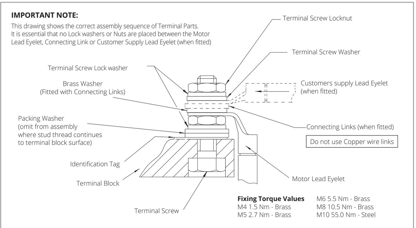
**FIXING ARRANGEMENT OF TERMINAL BLOCK**
