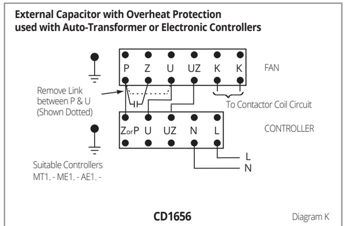
**WIRING DETAIL: SINGLE-PHASE DIRECT-DRIVE MOTOR WITH SPEED CONTROLLER**
